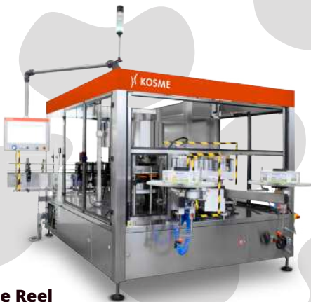
Kosme Reel Roll fed technology Exact container positioning by means of centring bell and centring plate Servo-controlled container plates for specially-shaped containers in the higher output range Hotmelt gluing unit with steel glue roller and adjustable glue scraper Operation with quick access to the user interface thanks to of individual transponders
